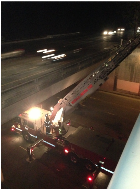
Moraga-Orinda Fire District ladder truck was used to raise personnel from Camino Pablo to trip breaker to de-energize power to the burning train car.
